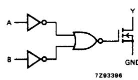
Fig.5 Logic diagram (one gate).
