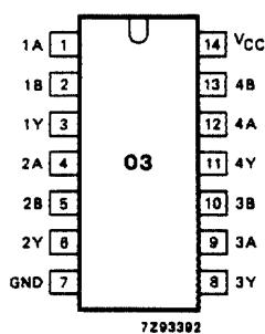
Fig.1 Pin configuration.
