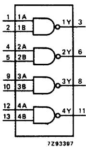
Fig.4 Functional diagram.
